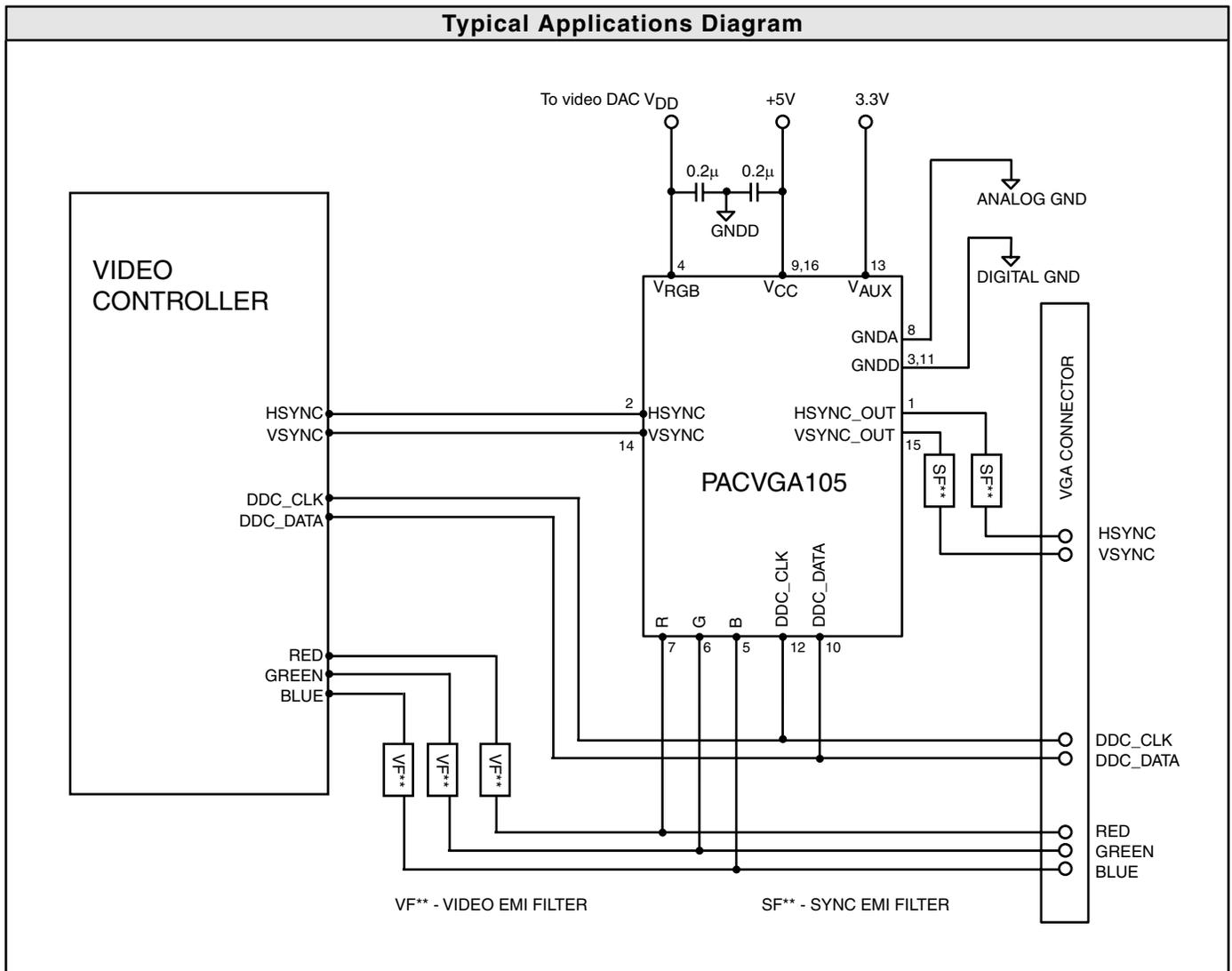
GND<sub>A</sub>, the negative voltage rail for the R,G,B diodes is not connected internally to GND<sub>D</sub>. GND<sub>A</sub> should ideally be connected to the ground of the video DAC IC. This will prevent any ground bounce caused by digital signals from injecting noise onto the R,G,B signals. Analog GND and digital GND will typically be connected on the pcb.
