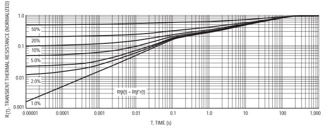
Figure 10. Thermal Response Junction to Ambient
