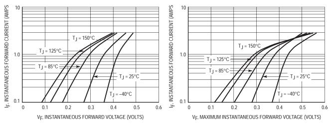
Figure 1. Typical Forward Voltage
