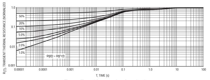
Figure 9. Thermal Response Junction to Lead
