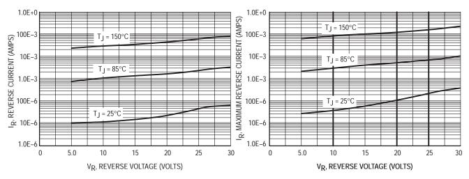
**Figure 3. Typical Reverse Current**
