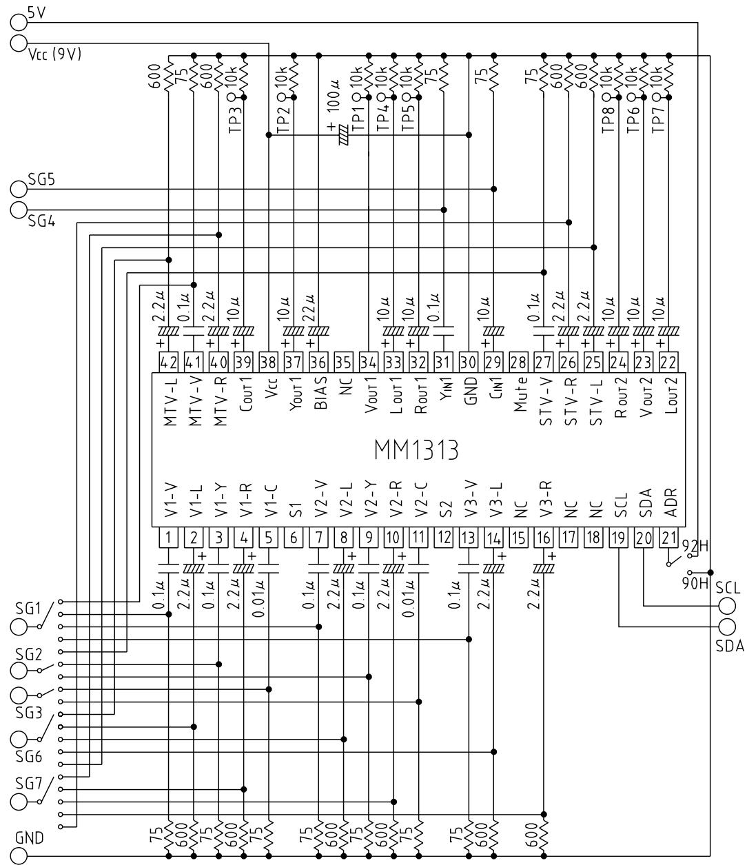
■ Measurement Circuit 2 (Crosstalk measurement)
