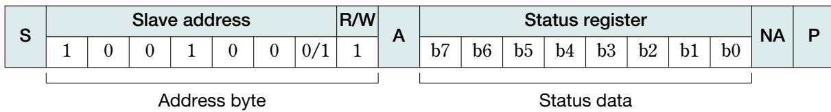
The data format is set as shown in the figure above. The first 7 bits in the address byte are allocated to the slave address, and the remaining 1 bit is allocated to the read/write bit. The read/write bit is set at 1 when using as a status register.
