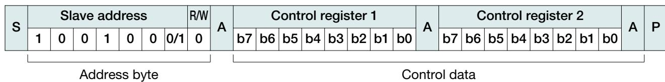
The data format is set as shown in the figure above. The first 7 bits in the address byte are allocated to the slave address, and the remaining 1 bit is allocated to the read/write bit. The read/write bit is set at 0 when using as a control register.
