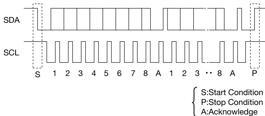
The I<sup>2</sup>C BUS is a BUS system developed by Philips for internal use in equipment. Data transmission is carried out by the two SDA and SCL lines, in byte units, with the MSB first from start condition.
