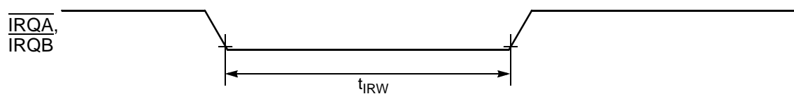
Figure 10-6 External Interrupt Timing (Negative-Edge Sensitive)
