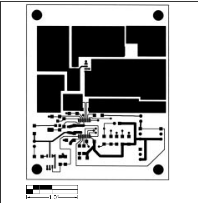
Figure 3. MAX745 EV Kit PC Board Layout—Component Side
