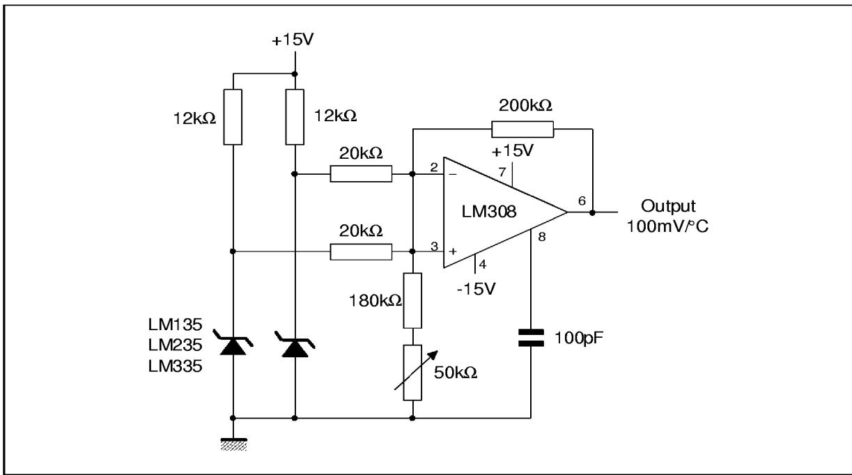
**THERMOCOUPLE COLD JUNCTION COMPENSATION**
