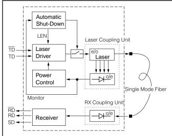
The receiver component converts the optical serial data into PECL compatible electrical data (RD and RDnot). The Signal Detect (SD, active high) shows whether an optical signal is present.
