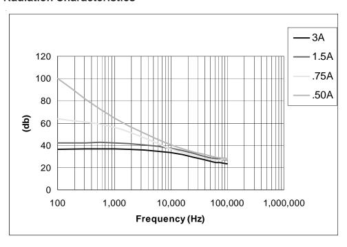
Fig 1. Ripple Rejection Vs Frequency
