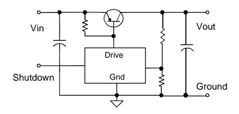
Fig 3. Simplified Schematic Circuit
