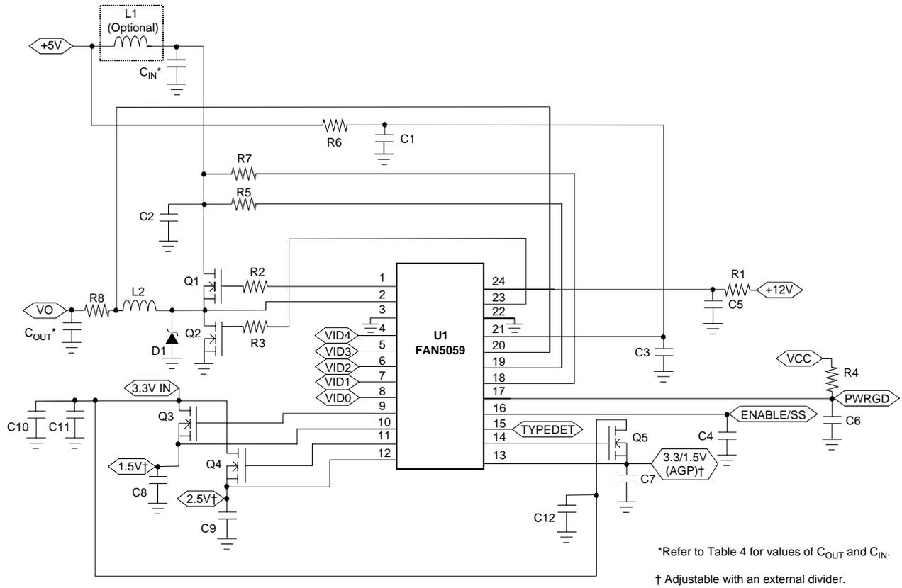
**Figure 2. Application Circuit for Coppermine/Camino Motherboards**
