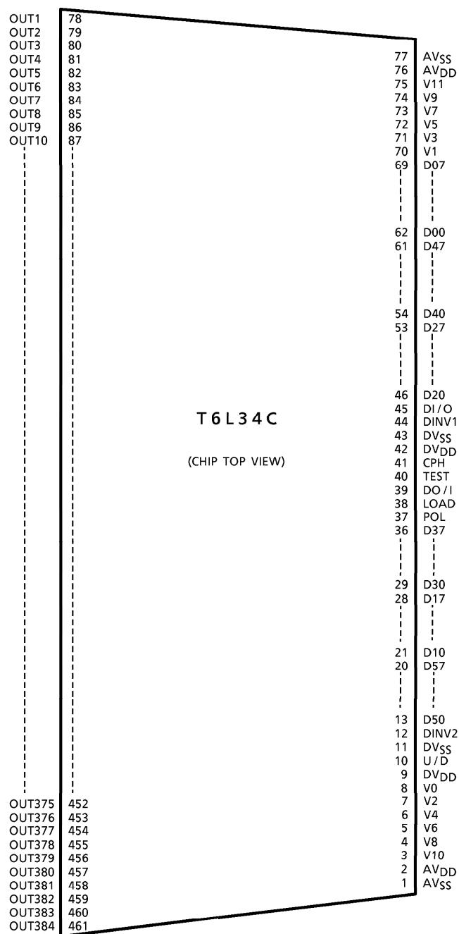
The above diagram shows the device's pin configuration only and does not necessarily correspond to the pad layout on the chip. Please contact Toshiba or our distributors for the latest TCP specification.
