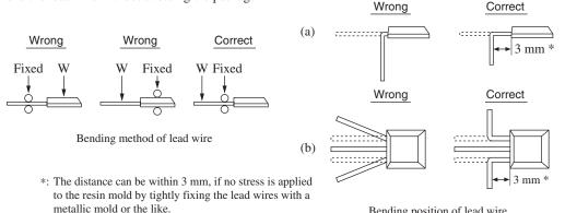
Bending position of lead wire
