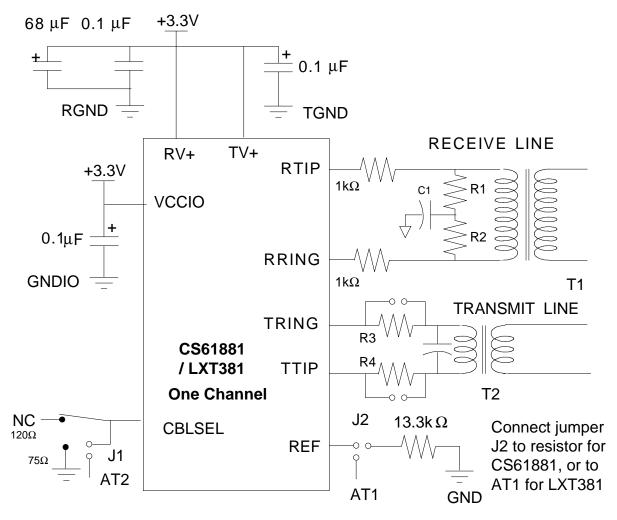
For CS61881, disconnect jumper J1 and set switch for cable type. For LXT381, set switch to NC and connect J1 to AT2.
