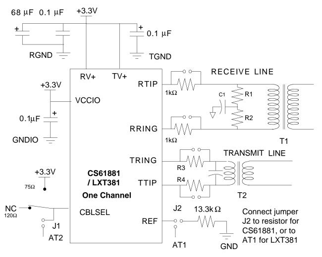
For CS61881, disconnect jumper J1 and set switch for cable type. For LXT381, set switch to NC and connect J1 to AT2.
