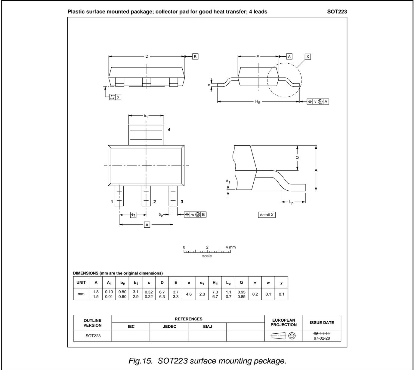
Fig. 15. SOT223 surface mounting package.
