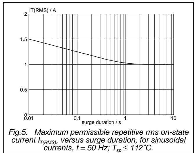
Fig. 5. Maximum permissible repetitive rms on-state current  $I_{T(RMS)}$ , versus surge duration, for sinusoidal currents,  $f = 50$  Hz;  $T_{sp} \leq 112^\circ\text{C}$ .
