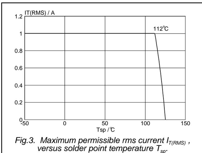
Fig. 3. Maximum permissible rms current  $I_{T(RMS)}$ , versus solder point temperature  $T_{sp}$ .
