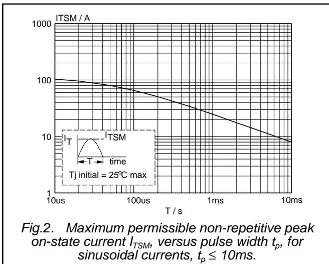
Fig. 2. Maximum permissible non-repetitive peak on-state current  $I_{TSM}$ , versus pulse width  $t_p$ , for sinusoidal currents,  $t_p \leq 10$  ms.
