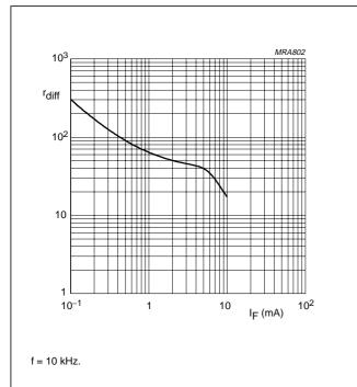
Fig.4 Differential forward resistance as a function of forward current; typical values.
