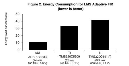
TMS320C5501 are both dual-MAC DSPs, only the ADSP-BF533 uses its dual-MAC capability on this benchmark. In the TMS320C5501, the two MAC units share an input—a restriction not imposed by most architectures. The TMS320C5501 is therefore limited to single-MAC operation on the filtering section of this benchmark. In contrast, the ADSP-BF533 uses both of its MAC units on this benchmark. As a result, the ADSP-BF53xx is significantly more efficient than the TMS320C5501 on this benchmark.
