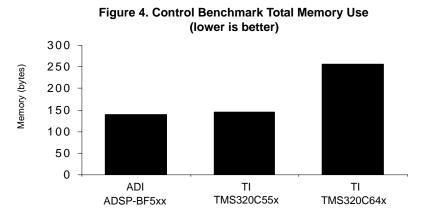
Control-oriented tasks usually constitute the bulk of an application's program memory requirements, but only a fraction of the application processing time. Thus, in control-oriented tasks, minimizing memory use is usually a more serious concern than maximizing execution speed.
