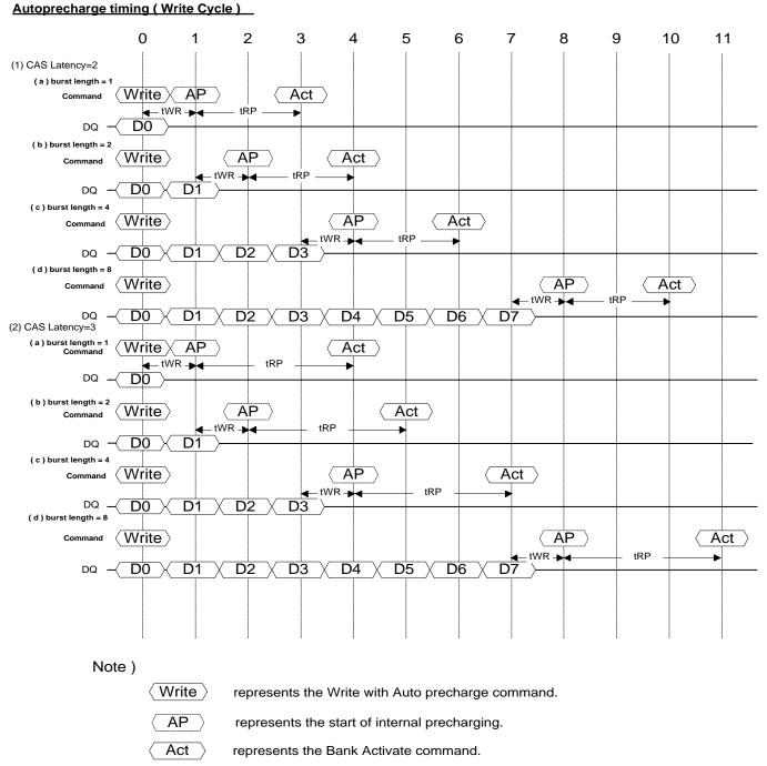
When the Auto precharge command is asserted, the period from Bank Activate command to the start of internal precgarging must be at least tRAS(min)
