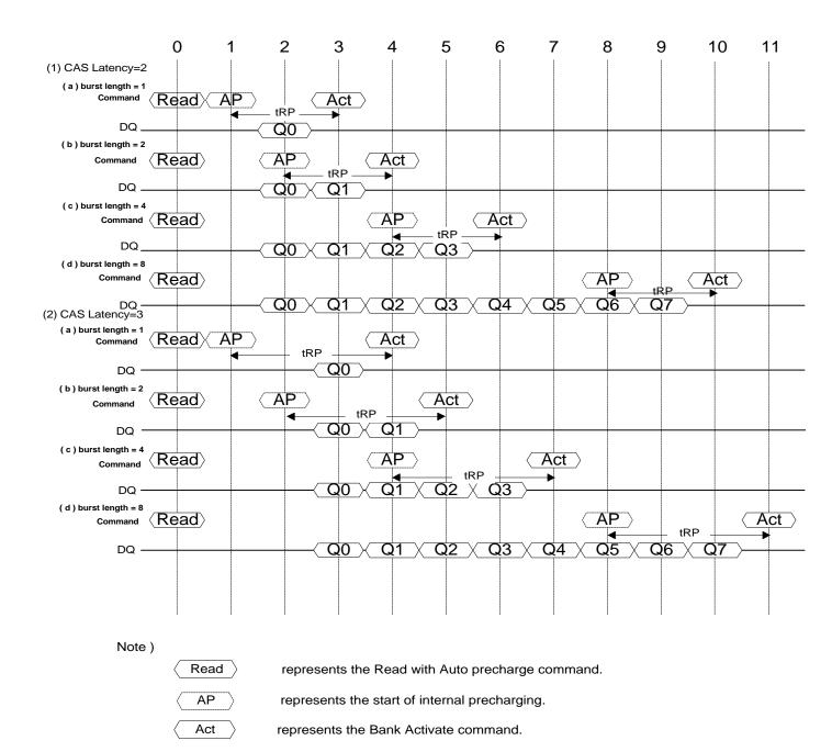
When the Auto precharge command is asserted, the period from Bank Activate command to the start of internal precgarging must be at least tRAS(min).
