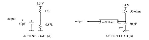
7. Transition times are measured between  $V_{\mbox{\tiny IH}}$  and  $V_{\mbox{\tiny IL}}.$
