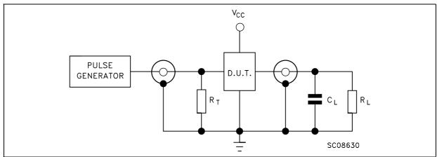
$C_L = 5/35 pF$  or equivalent (includes jig and probe capacitance)  $R_L = 50 \Omega$  or equivalent  $R_T = Z_{OUT}$  of pulse generator (typically  $50 \Omega$ )
