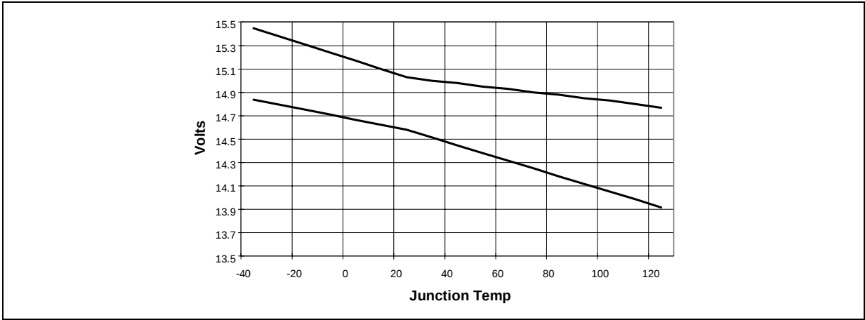
Figure 3. Set-Point Voltage vs. Thermistor Temperature, T j = 90°C (Not guaranteed by testing, depending on NTC characteristics)
