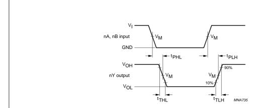
For HC2G:  $V_M$  = 50%;  $V_I$  = GND to  $V_{CC}$ . For HCT2G:  $V_M$  = 1.3 V;  $V_I$  = GND to 3.0 V.
