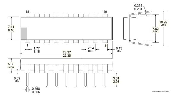
NOTES: 1. Exact body and lead configuration at vendor's option within limits shown.2. Lead spacing tolerance is non-cumulative.3. Lead thickness is measured at seating plane or below.
