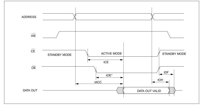
\* If  $\overrightarrow{CE}$  is kept low and address pins are kept at constant during power-up, the time period between  $\overrightarrow{OE}$  going low and data out valid shoud be treated as tACC instead of tOE.
