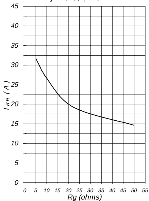
Fig.18 - Typical Diode I_{RR} vs R_g T_J=125^\circ\text{C}; I_F=20\text{A}
