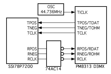
All other connections to the PM8313 D3MX and SSI78P7200 should be made according to the latest issues of the respective datasheets.
