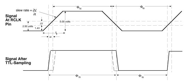
In Figure 1,  $\Delta V$  is the difference between the CMOS and TTL nominal switching voltage levels;  $\Delta t$  is the time difference between the CMOS and TTL nominal
