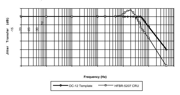
Conclusion: Jitter Transfer failed. Peaking of about 4dB at 110kHz observed.
