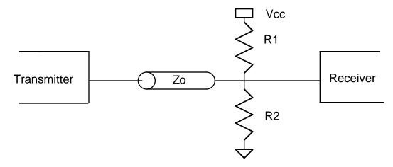
The resistors R1 and R2 in parallel must equal Zo and the voltage at the input must pull the output of the transmitting gate to VBB Volts. Working out the equations for PECL +5 Volt supply for Vcc gives:
