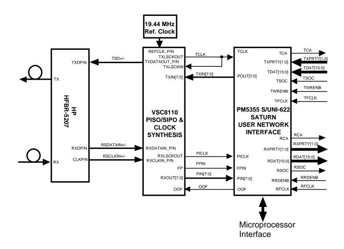
Figure 1. Block Diagram of 622 SONET/ATM Core.
