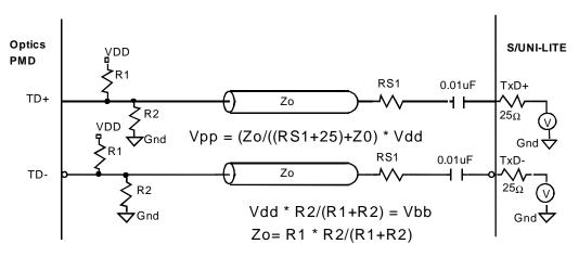
Notes: Vpp is minimum input swing required by the optical PMD device. Vbb is the switching threshold of the PMD device (typically Vdd - 1.3 volts) Vpp is Voh - Vol (typically 800 mVolts) For Zo = 50  $\Omega$ , R1=67  $\Omega$ , R2 = 192.3  $\Omega$ , RS1=237 $\Omega$
