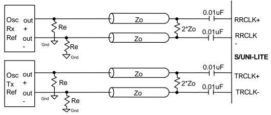
The value of Re is dependent on the signal trace characteristic impedence and the ECL or PECL supply voltage (-4.5 V, + 5 V). Values in the range of 200-330  $\Omega$  are recommended
