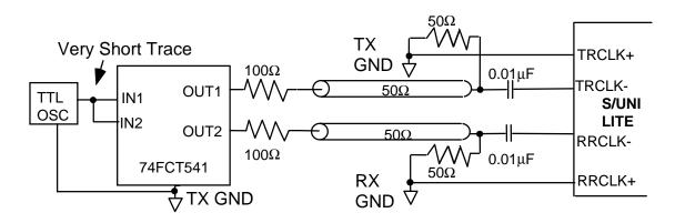
The TTL oscillator should be placed as close to the buffer as possible as it is unterminated. The TTL oscillator is used to match the 74FCT541's TTL input level in order to avoid duty cycle distortion caused by differences in output levels and input switching thresholds.
