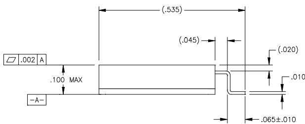
Molybdenum pad with Ni plating and Sn63 solder finish
