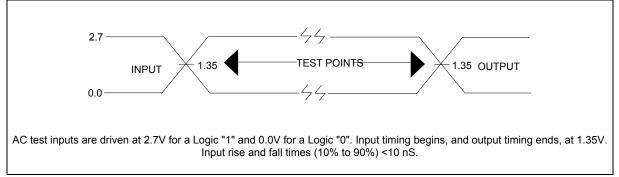
Figure 12. Transient Input/Output Reference Waveform for VDD = 2.7V to 3.6V
