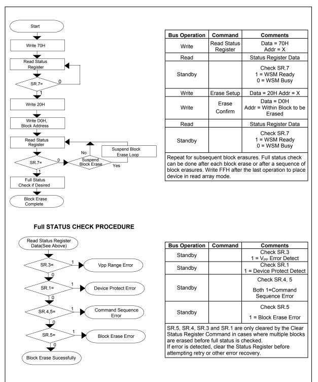
Figure 5. Automated Block Erase Flowchart
