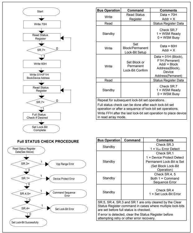
Figure 10. Set Block and Permanent Lock-Bit Flowchart
