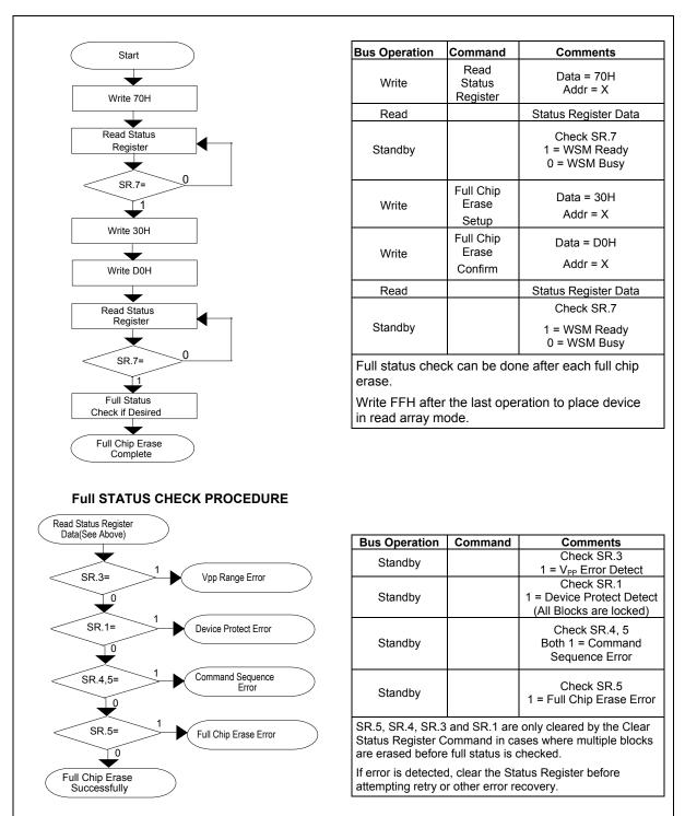
Figure 6. Automated Full Chip Erase Flowchart
