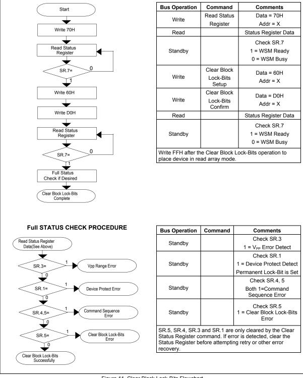
Figure 11. Clear Block Lock-Bits Flowchart
