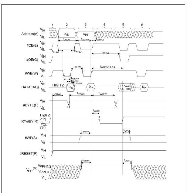
Figure 16. AC Waveform for #WE-Controlled Write Operations
