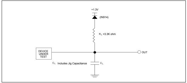
Figure 13. Transient Equivalent Testing Load Circuit
