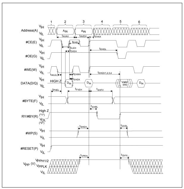
Figure 17. AC Waveform for #CE-Controlled Write Operations
