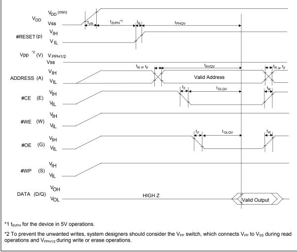
Figure 19. AC Timing at Device Power-up
