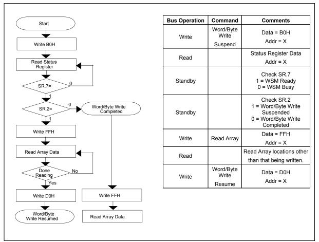
Figure 9. Word/Byte Write Suspend/Resume Flowchart
