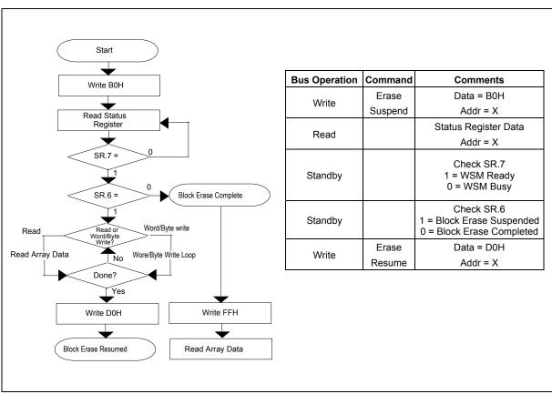
Figure 8. Block Erase Suspend/Resume Flowchart
