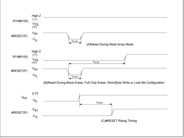
Figure 18. AC Waveform for Reset Operation
