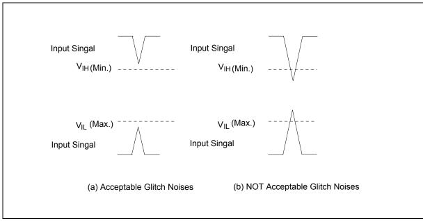
Figure 20. Waveform for Glitch Noises
