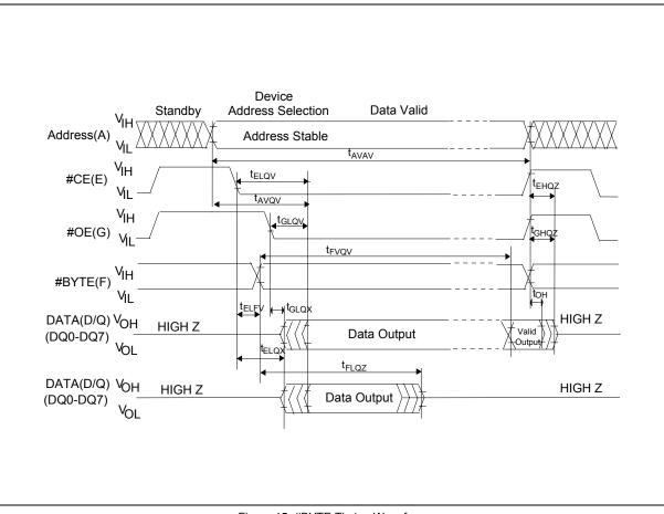
Figure 15. #BYTE Timing Waveform
