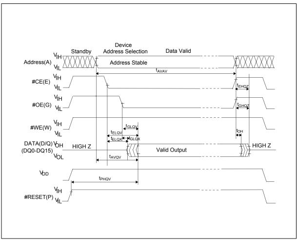
Figure 14. AC Waveform for Read Operations
