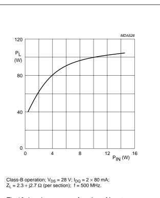
Fig.10 Load power as a function of input power, typical values.
