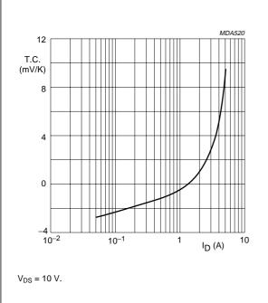
Fig.4 Temperature coefficient of gate-source voltage as a function of drain current, typical values per section.
