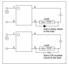
2) If spike voltages generated at the load are limited with a clamp diode and the circuit wires are long, spike voltages will occur by inductance.
