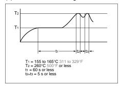
temperature may increase excessively. Check the temperature under mounting conditions.
