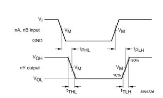
For 74HC2G08:  $V_M$  = 50%;  $V_I$  = GND to  $V_{CC}$ . For 74HCT2G08:  $V_M$  = 1.3 V;  $V_I$  = GND to 3.0 V.
