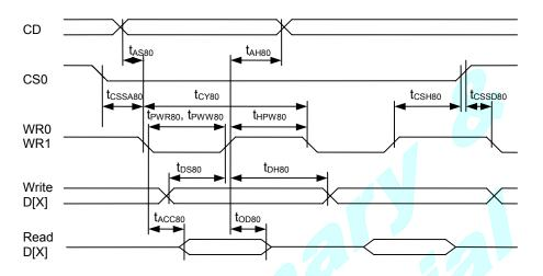
Parallel Bus Timing Characteristics (for 8080 MCU)
