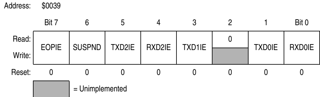
Figure 9-16. USB Interrupt Register 0 (UIR0)
