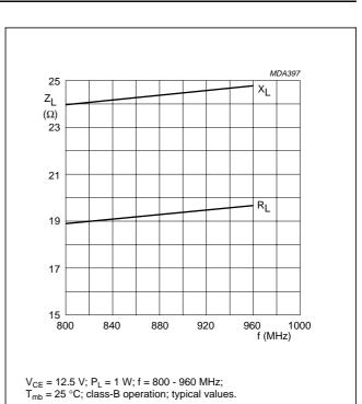
Fig.10 Load impedance (series components).
