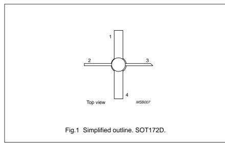
PRODUCT SAFETY This device incorporates beryllium oxide, the dust of which is toxic. The device is entirely safe provided that the BeO disc is not damaged.
