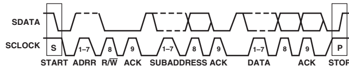
Figure 13. Bus Data Transfer
