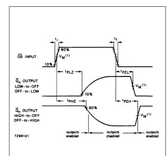
(1) HC :  $V_M$  = 50%;  $V_I$  = GND to  $V_{CC}$ . HCT:  $V_M$  = 1.3 V;  $V_I$  = GND to 3 V.
