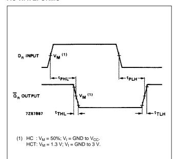
Fig.6 Waveforms showing the data input  $(D_n)$  to output  $(\overline{Q}_n)$  propagation delays and the output transition times.
