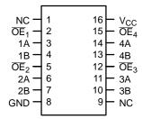
Figure 2. Pin Assignment for QSOP
