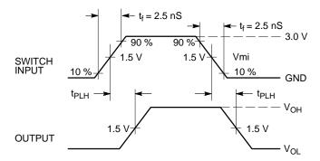
Figure 5. Propagation Delays
