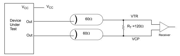
Figure 1. Differential Signal Using Direct Termination Resistor
