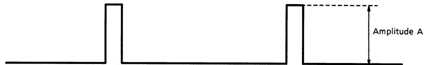
Fig.C Test signals for TA1310ANG chroma, color difference, and Y stage
