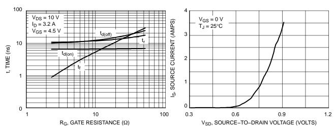
Figure 9. Resistive Switching Time Variation versus Gate Resistance
