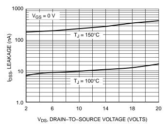
Figure 6. Drain-to-Source Leakage
