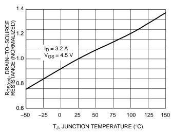
Figure 5. On–Resistance Variation with Temperature
