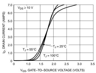
Figure 2. Transfer Characteristics
