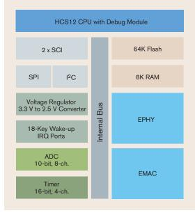
> 25 MHz operation at 3.3 V for 40 nsec minimum instruction cycle time
