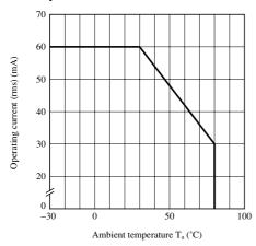
Fig.2 Forward Current vs. Ambient Temperature
