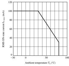
Fig.3 Operating Current vs. Ambient Temperature
