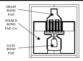
DIE SIZE: 14.2X13.0 mils (360x330  $\mu m)$  DIE THICKNESS: 3.9 mils (100  $\mu m)$  BONDING PADS: 1.9X1.9 mils (50x50  $\mu m)$
