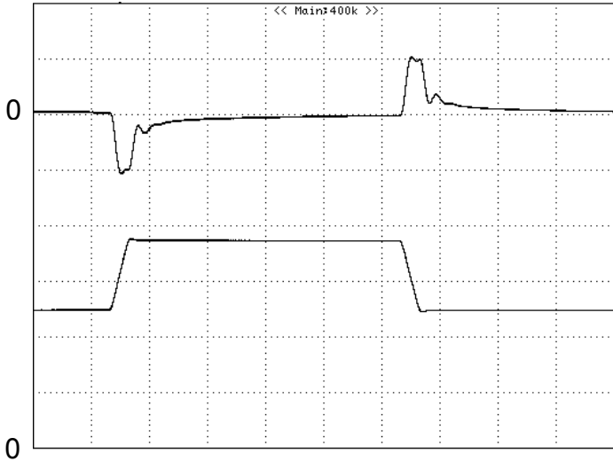
Figure 8: Output voltage response to step-change in load current (75%-50%-75% of I_o , max; di/dt = 0.1A/\mu s ). Load cap: 10\mu F tantalum capacitor and 1\mu F ceramic capacitor. Top Trace: V_{out} (50mV/div, 200us/div), Bottom Trace: I_{out} (5A/div). Scope measurement should be made using a BNC cable (length shorter than 20 inches). Position the load between 51 mm to 76 mm (2 inches to 3 inches) from the module
