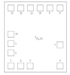
CHIP SIZE: 900  $\times$  1020  $\mu$  m<sup>2</sup> SUBSTRATE: V<sub>DD</sub>
