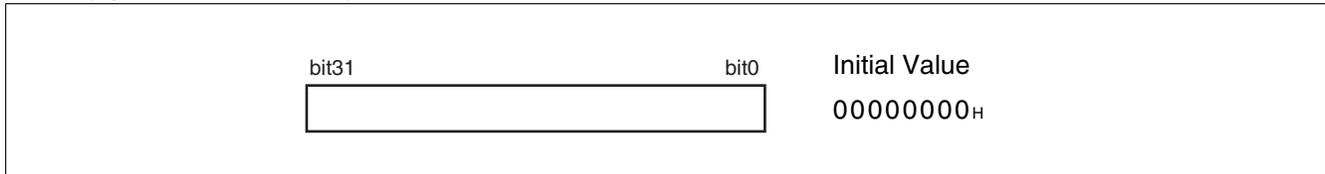
The SSP is the system stack pointer and functions as R15 when the S flag is “0”. The SSP can be explicitly specified. The SSP is also used as the stack pointer that specifies the stack for saving the PS and PC when an EIT event occurs. The initial value after a reset is 00000000H.
