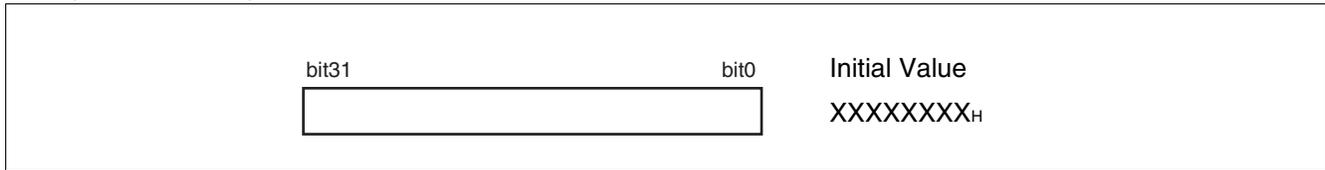
The return pointer contains the address to which to return from a subroutine. When the CALL instruction is executed, the value in the PC is transferred to the RP. When the RET instruction is executed, the value in the RP is transferred to the PC. The initial value after a reset is indeterminate.
