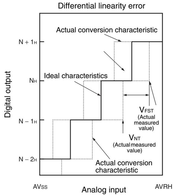
$$\text{Linearity error of digital output } N = \frac{V_{NT} - \{1 \text{ LSB}' \times (N - 1) + V_{OT}\}}{1 \text{ LSB}'} \text{ [LSB]}$$
