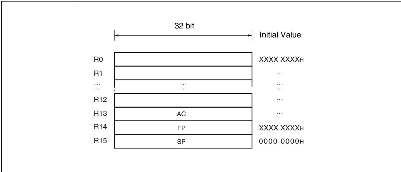
Registers R0 to R15 are general purpose registers. The registers are used as the accumulator and memory access pointers for CPU operations.
