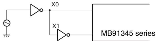
[The STOP mode (oscillation stop mode) cannot be used.]
