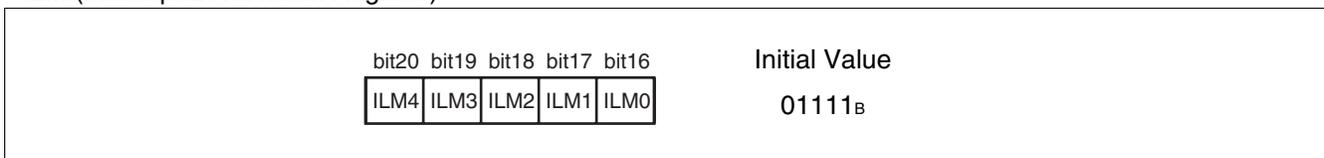
This register stores the interrupt level mask value. The value in the ILM register is used as the level mask. Initialized to “15” (01111<sub>B</sub>) by a reset.
