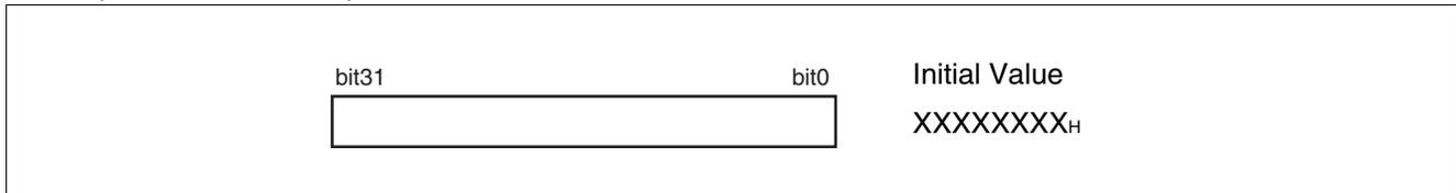
The USP is the user stack pointer and functions as R15 when the S flag is “1”. The USP can be explicitly specified. The initial value after a reset is indeterminate. This pointer cannot be used by the RETI instruction.
