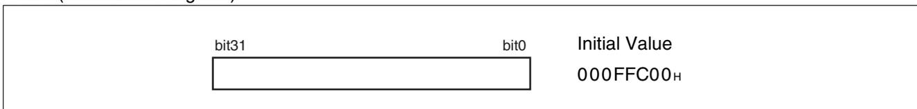
The table base register contains the start address of the vector table used for servicing EIT events. The initial value after a reset is 000FFC00<sub>H</sub>.
