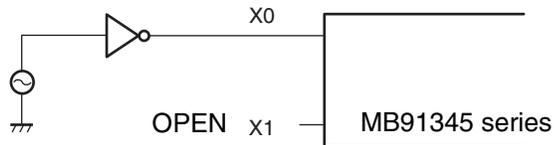
Note : The X1 pin must be designed to have a delay within 15 ns, at 10 MHz, from the signal to the X0 pin.
