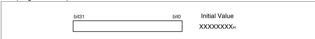
The program counter contains the address of the instruction currently being executed. The initial value after a reset is indeterminate.
