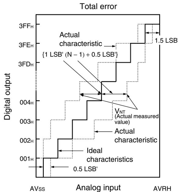
$$1 \text{ LSB}' (\text{ideal value}) = \frac{\text{AVRH} - \text{AVSS}}{1024} [\text{V}]$$
