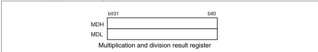
These registers hold the results of a multiplication or division. Each of them is 32-bit long. The initial value after a reset is indeterminate.
