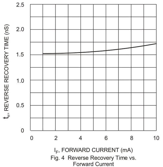
Fig. 4 Reverse Recovery Time vs. Forward Current
