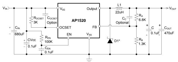
Note:  $V_{OUT} = V_{FB} x (1+R_A/R_B)$  $R_B=0.7K\sim5K \text{ ohm}$
