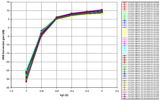
XUI009-BD\_5samples: USB Conv Gain (dB), I<sub>d1</sub> & IIP<sub>3</sub> (dBm) vs. Vg1 (V)
