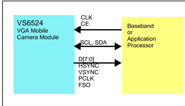
Figure 2. Block diagram
