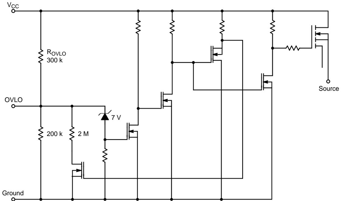
Figure 18. Equivalent Overvoltage Lockout Circuit
