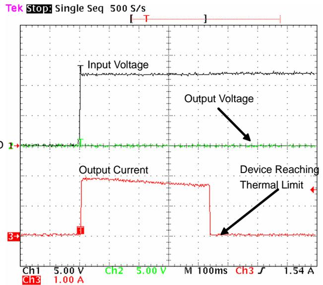
Figure 10. Turn-on Waveforms for Shorted Output, Latchoff Device
