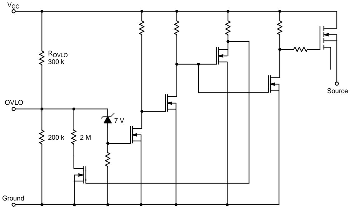
Figure 18. Equivalent Overvoltage Lockout Circuit
