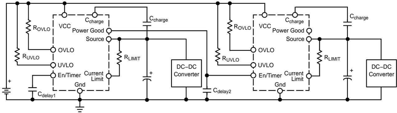
Figure 13. Turn-on Sequencing Using Power Good Signal
