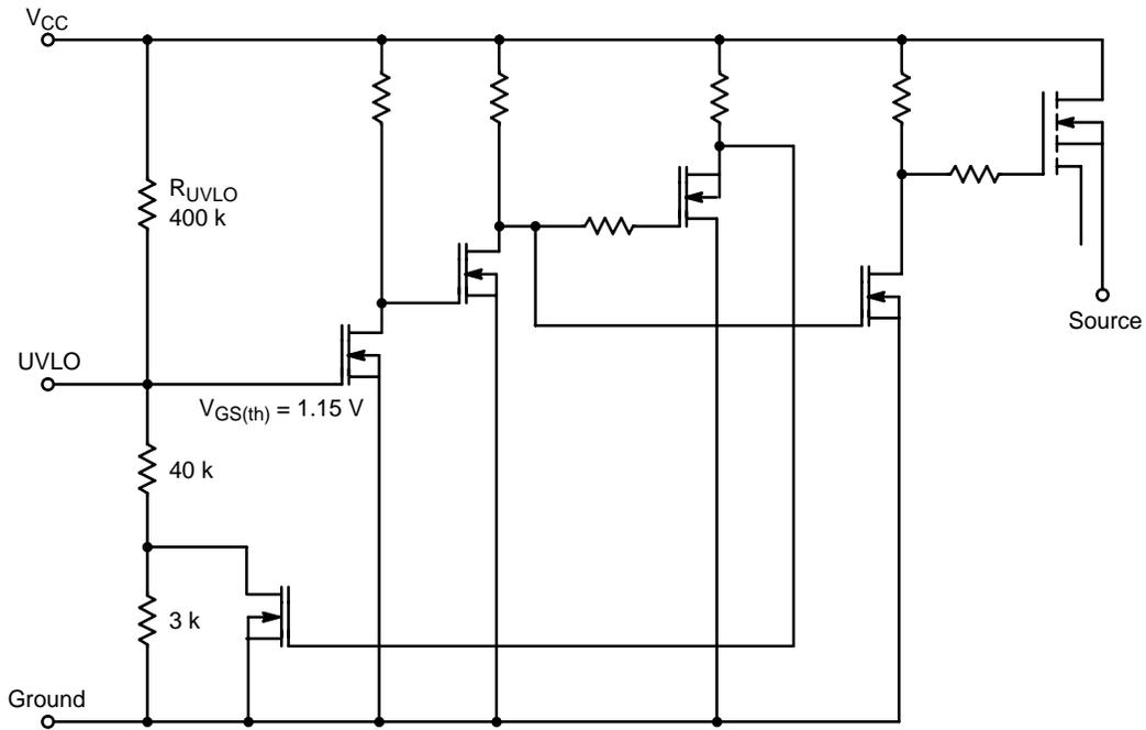
Figure 17. Equivalent Undervoltage Lockout Circuit
