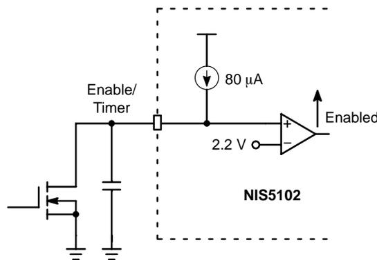
Figure 16. Enable/Timer Circuit
