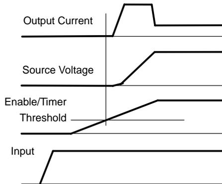
Figure 2. Timing Diagram for External Enabled Delay
