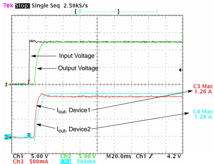
Figure 15. Turn-on Waveforms for Parallel Operation
