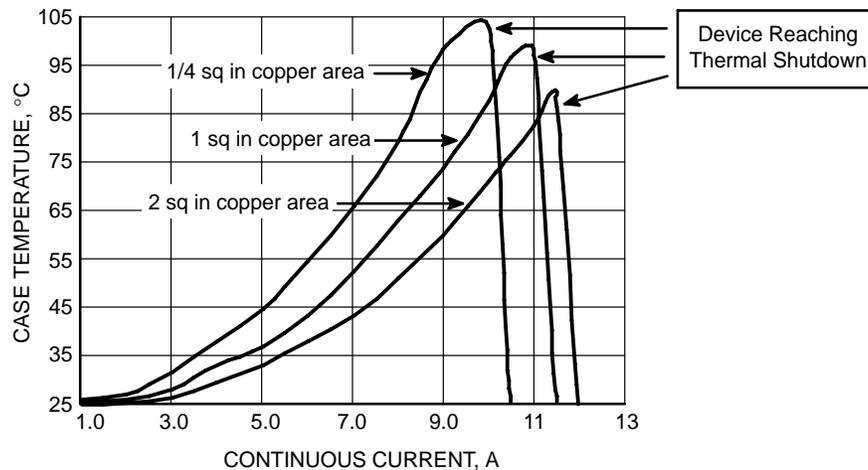
**Figure 7. Continuous Current vs. Case Temperature**
