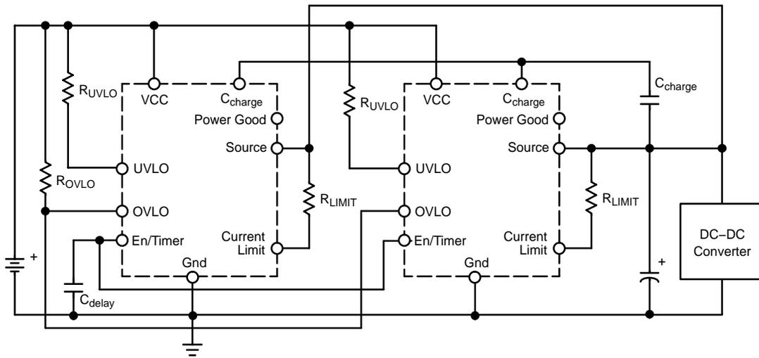
Figure 14. Parallel Operation / Simultaneous Turn-on and Shutdown
