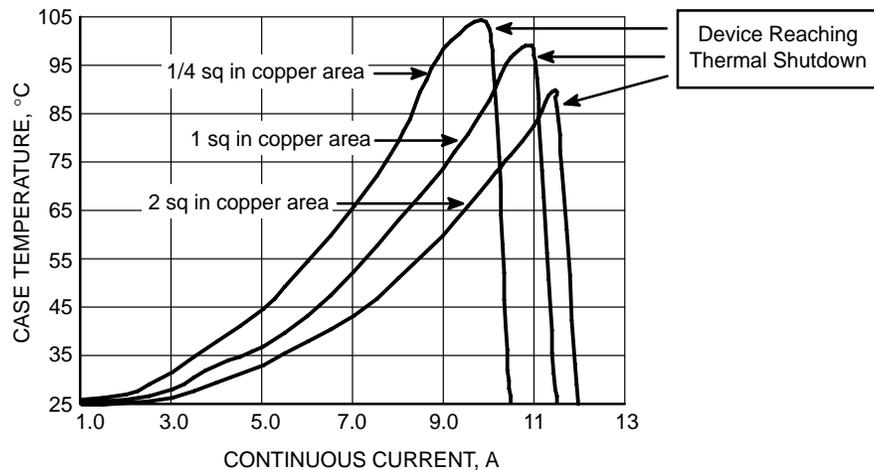
**Figure 7. Continuous Current vs. Case Temperature**
