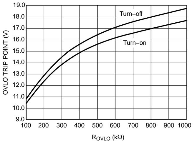
**Figure 4. OVLO Adjustment**
