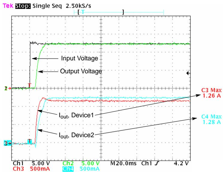
Figure 15. Turn-on Waveforms for Parallel Operation
