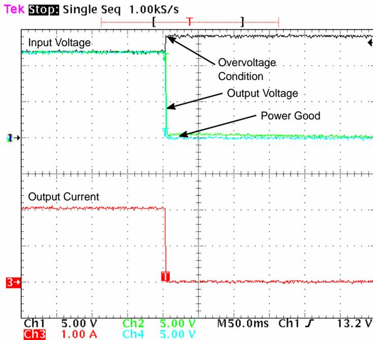
Figure 12. Device Response During an Overvoltage Condition
