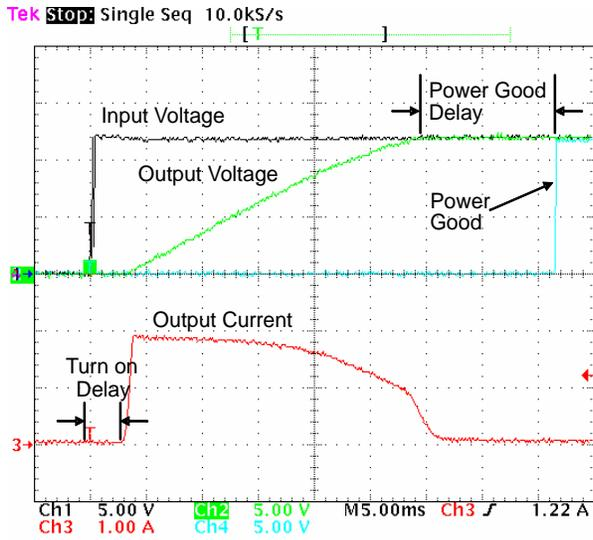
Figure 9. Turn-on Waveforms for 3300  $\mu\text{F}$  Load Capacitors
